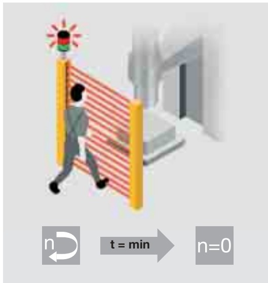
Should a hazardous event occur, the PSS programmable safety and control systems react particularly quickly.
