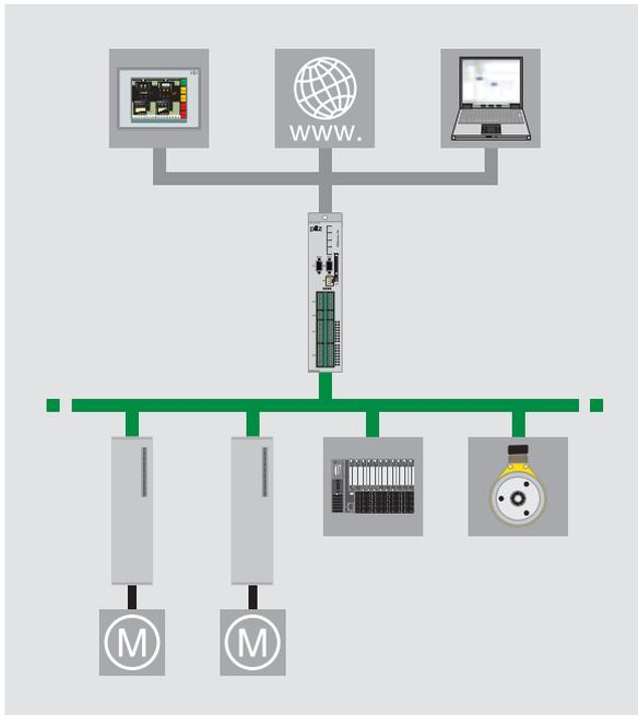
Control systems PMCprimo 16+ and PMCprimo Drive are used for all types of motion and control functions. They consist of PLC and motion technology. They perform the automation within a plant, including management of all the movements for a large number of physically separate servo axes.
